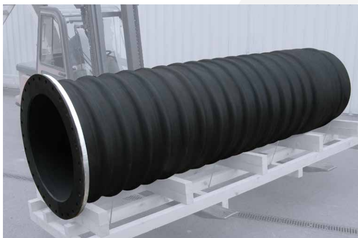
Wear-proof hose with embedded support rings for water and slag removal in a steel mill NB 900, wall thickness 80 mm, length 3900 mm
