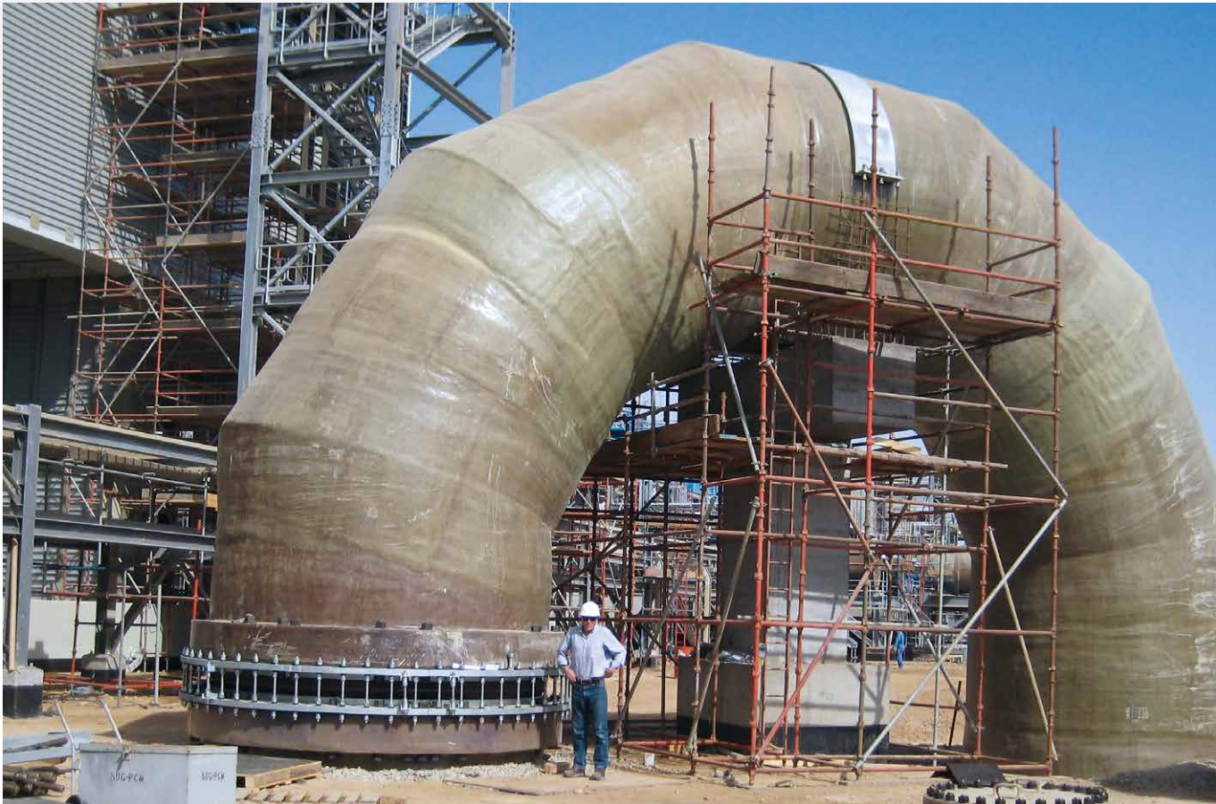
Large bore lateral rubber expansion joint, type U110M GRP pipe DN 3600 of a utility plant work-shop hydraulic test at 13 bar
