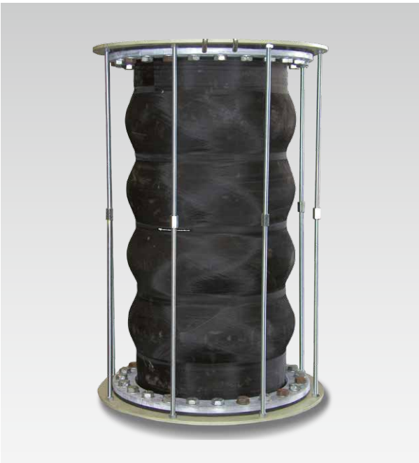
Wear-proof hose for water and sand conveyance on a dredger, at pressure test NB 580, 3 bar
