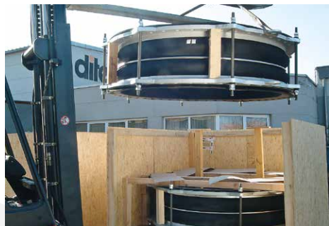
Lateral expansion joints type U121E for a marine supply line NB 2000, +2 / -1 bar ▶ page 65
