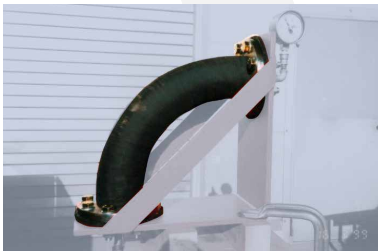
Rubber bend in pressure test NB 100, 40 bar
