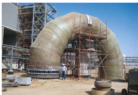
Large bore lateral rubber expansion joint, type U110M GRP pipe NB 3600 of a utility plant work-shop hydraulic test at 13 bar ▶ page 155
