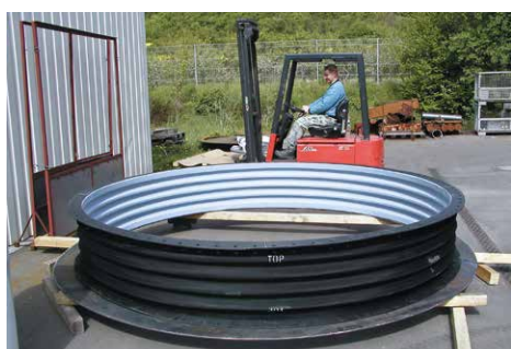
Universal expansion joint, type U142A with PTFE lining for a sulphuric acid reclamation plant NB 2800, -0.15 bar, 80 °C ► page 79
