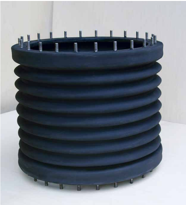
Expansion bellows with embedded steel flanges and stay bolt for a radial-flow scrubber NB 780, -0.2 bar
